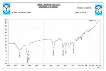
Figure 3 FT IR spectrum of essential oil (leaf oil) from C. hystrix leaf
